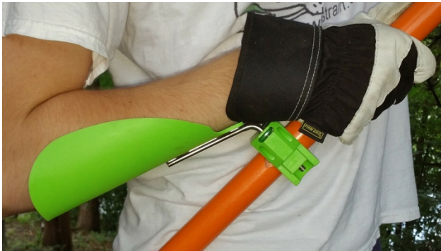
Figure 15 Long-Handled Tool Leverage Booster (Why Strain)
