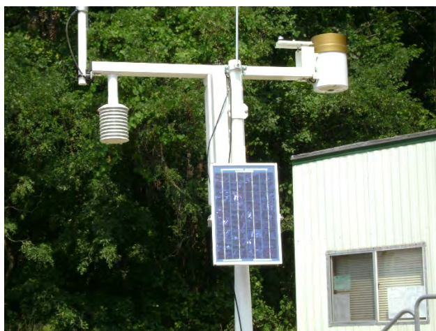
Figure 10. Onsite weather stations can provide potential ET data to help determine irrigation needs.
