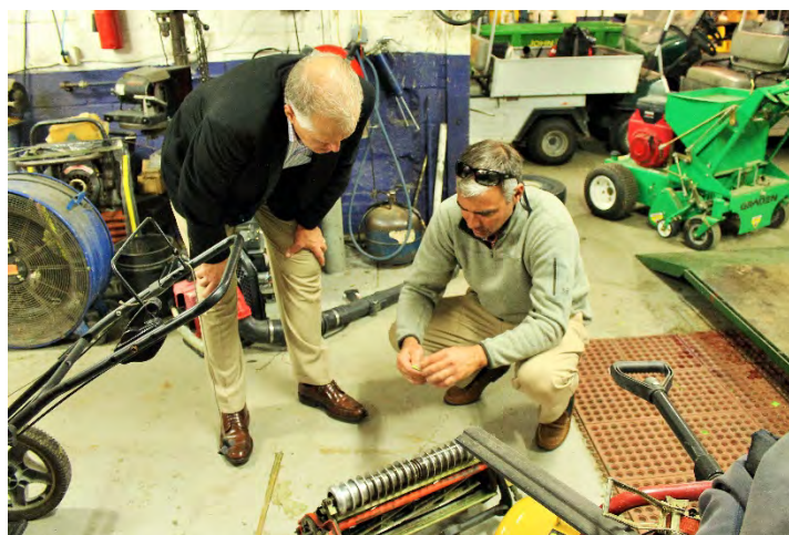
Figure 29. Checking mower reel sharpness at Belle Haven Country Club.
