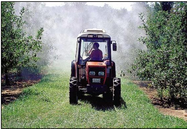
Figure 1. An airblast sprayer creates many fine droplets prone to drift.
