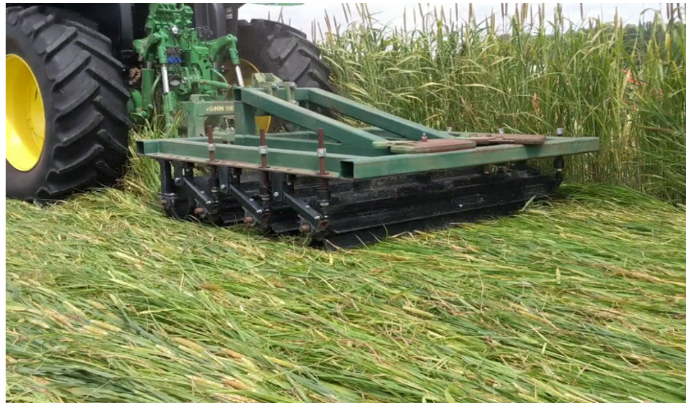
Figure 2. Cover crop being terminated with a roller crimper. This specific roller crimper has a roller followed by three spring-loaded crimpers.
