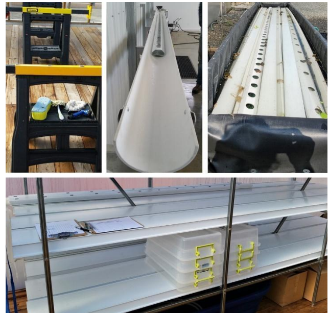
Figure 4. Methods for cleaning and sanitizing NFT channels: plastic sawhorses (top left); a large PVC pipe cut in half for placing channels sprayed with a pressure washer (top middle); a plastic-lined trough for soaking dirty channels (top right); and sanitized channels stored on a large shelving unit (bottom). (Amber Vallotton, Virginia Cooperative Extension)
